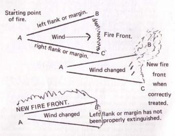
On change of wind, A TO B becomes the new fire front. If these smouldering spots had been extinguished before the wind changed, a small point at B only would constitute the front.
