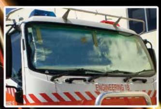
RADIANT HEAT SHIELDS - RFS
